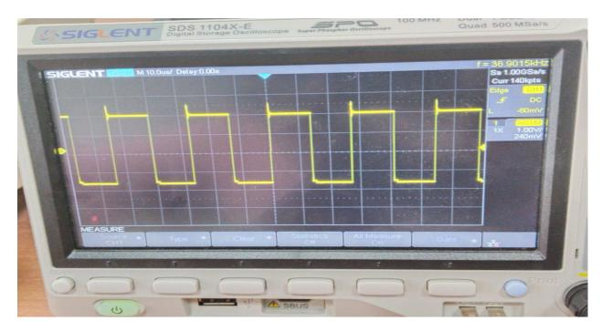
3. When the signal is not transmitted by the ir sensor the at the receiving end the voltage level is set to tsop1738 and look like :
